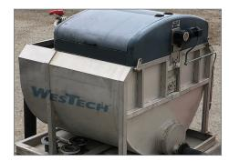
Once the underflow return activated sludge (RAS) and influent flow was set, only one operator was needed. One or two tanks were cleaned per day, taking approximately 45 minutes to an hour to clean one tank. Outside of cleaning, maintenance was not frequently needed. For redundancy, one more unit than necessary was added to allow for full treatment capacity while cleaning took place. In this case, four units were required, but five units were at the site.
