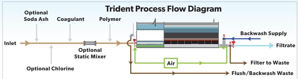
**The Trident provides flocculation, clarification, and filtration within a single tank.**
